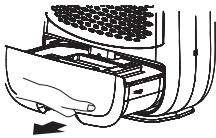
Pull water tank out
