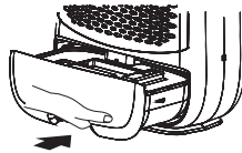
Refit the cover and restore the water tank into position
